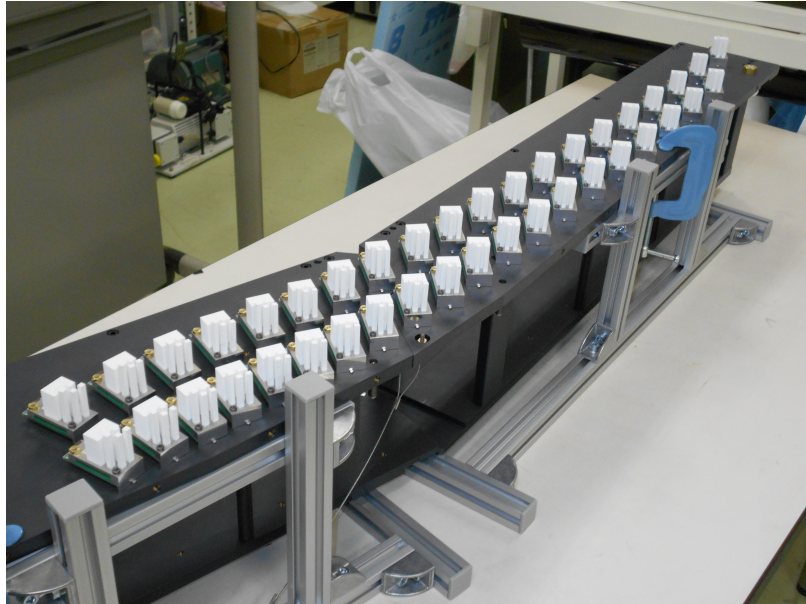
Fig.3. Photograph of the detector case of the tagger with all the counter units mounted on it.
