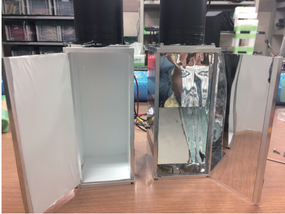
Fig.4. Photograph showing the insides of the detector frames of AC1 (right, mirror reflection) and AC2 (left, diffused reflection)
