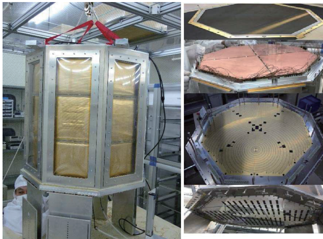
Fig.1. (left) The picture of developed TPC. (right) Gating wire, GEM, readout pad and conversion connector from the top picture.
