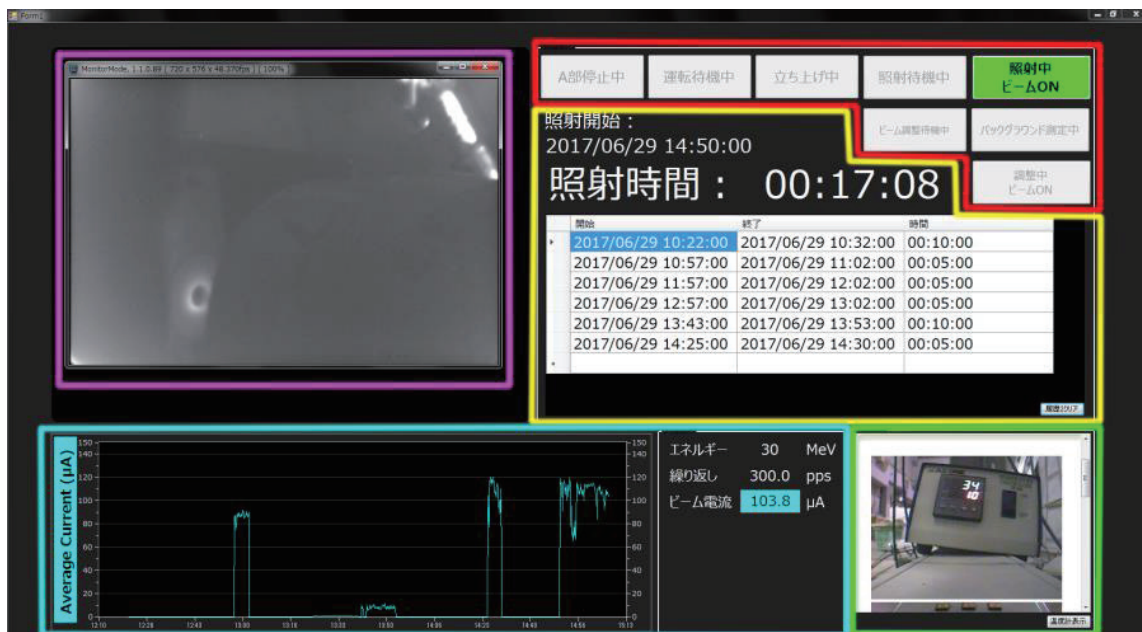
Fig.3. Operation status display. Current state in the operation sequence (red). History of the average beam current for 3 hours (cyan). Irradiation log in chronological order (yellow). Irradiation-position-monitor (magenta). Temperature indicator of water used for target cooling (green).
