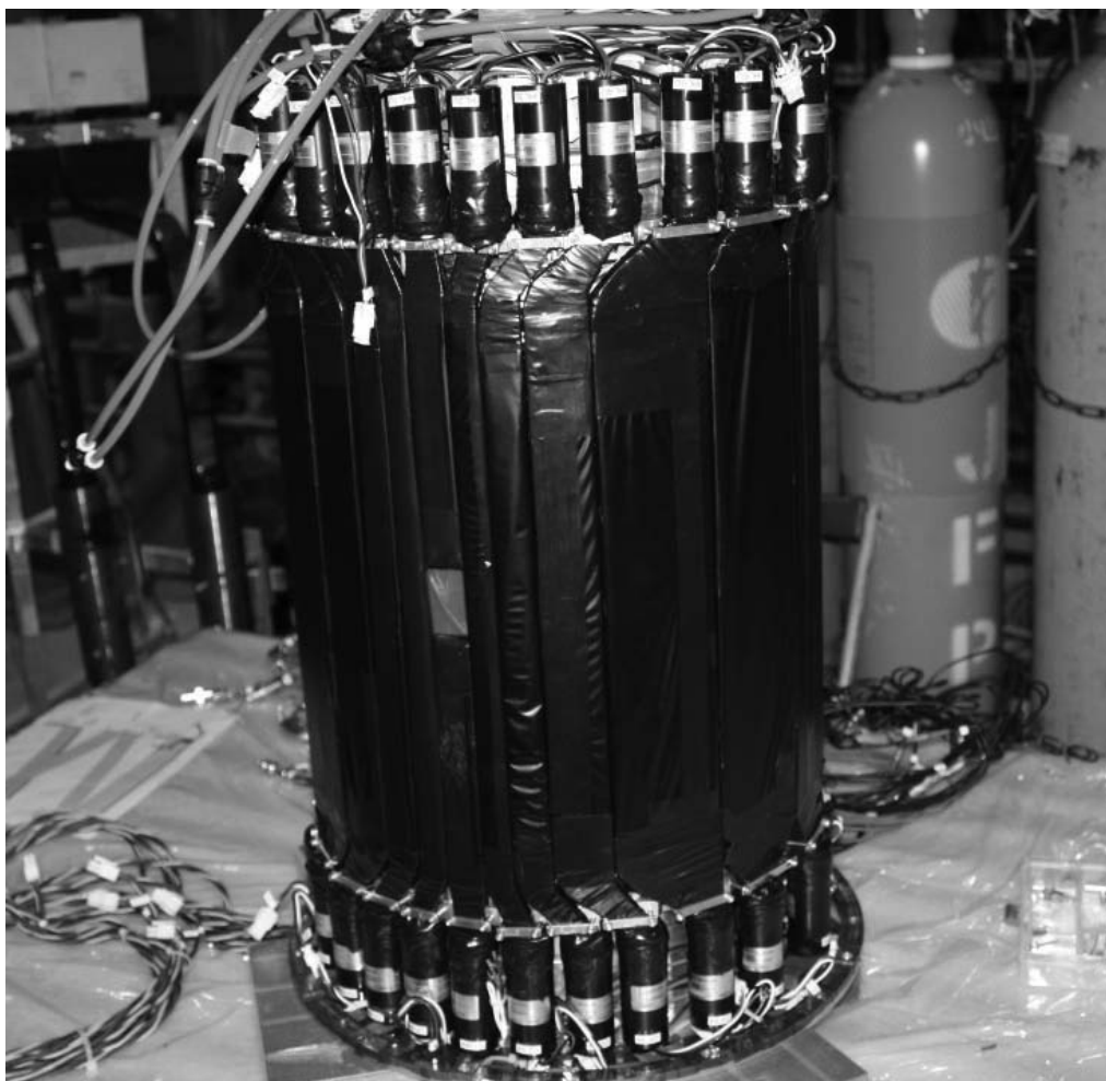
Fig.5. Picture of IH viewed from downstream side. The counters are mounted on VDC body. The PMT's are connected both edge of the scintillator, excepting 1L and 1R. Those have only one side read-out to avoid hit of photo beam.
