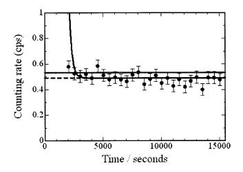
Fig.2. Time variation of the counting rate for photons emitted from <sup>229m</sup>Th HNO<sub>3</sub> solution sample grown for 17 hours in the 9M HCl.
