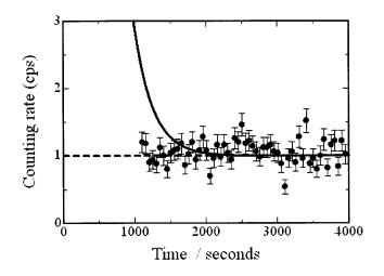
Fig.1. Time variation of the counting rate for photons emitted from <sup>229m</sup>Th HNO<sub>3</sub> solution sample grown for 2 hours in the 9M HCl.
