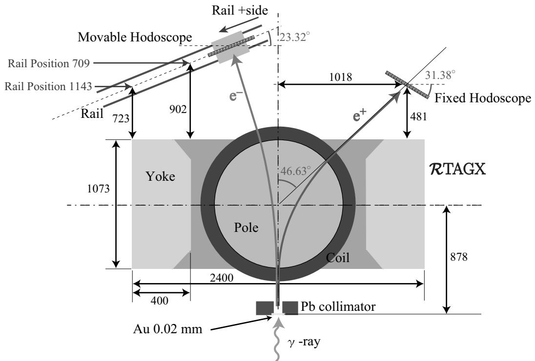
Fig.1. Experimental setup for the energy calibration of STB-Tagger II. The  $e^+e^-$  pairs are generated in the interaction of incident photons with a Au foil, and are detected by a fixed scintillating fiber hodoscope and a movable one.
