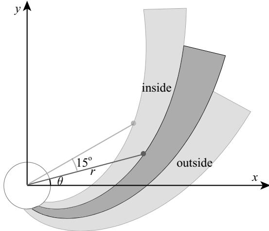
Fig.1. Spiral-shaped scintillators. The side curve of each plastic scintillator is represented as  $r = \exp\{b(\theta + \theta_0)\}$  in the polar coordinate system. The phase difference between adjacent scintillators is  $15^\circ$ .
